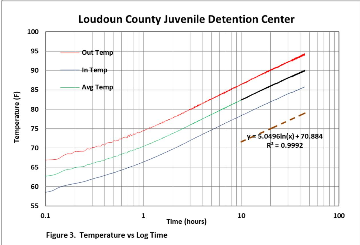
The calculated line-source model temperature at the borehole edge is also shown by the dashed line. The difference between the model bore-wall temperature and the average loop temperature, divided by the power input per foot yields the Borehole Thermal Resistance.
